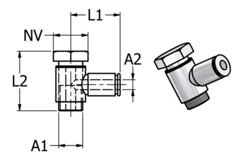
Ext. hose diameter A2 = 5L1 = 19 L2 = 17.5 NV = 8 Thread A1 = M5
